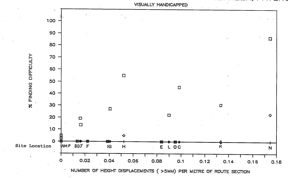
Fig 3.16 ASSESSMENT OF HEIGHT DIFFERENCES BETWEEN, PAVERS
