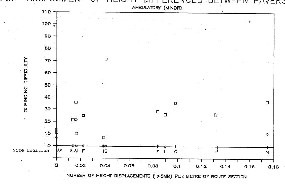
Fig 3.17 ASSESSMENT OF HEIGHT DIFFERENCES BETWEEN PAVERS
