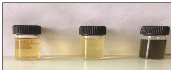
Fig. 1 — (A) C. sativum leaf extract; (B) 0.01M ferrous sulphate; and (C) Synthesized iron oxide nanoparticles
