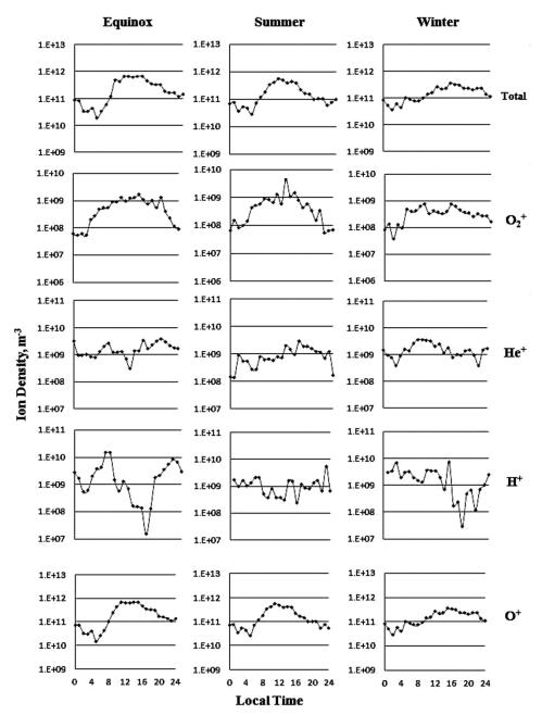
Fig. 2 — The ion density distribution with respect to local time over Indian region at an altitude of ~ 500 km during the medium solar activity period as measured by SROSS-C2 for three seasons.
