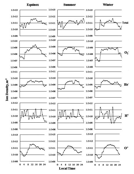
Fig. 1 — The ion density distribution with respect to local time over Indian region at an altitude of  $\sim$  500 km during the low solar activity period as measured by SROSS-C2 for three seasons.
