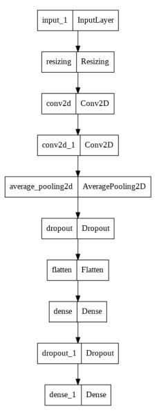
Figure 3. CNN architecture
