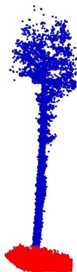
Fig. 4. The individual output from Cloth Simulated Filter (CFS) algorithm. The ground points are red and off-ground points blue.
