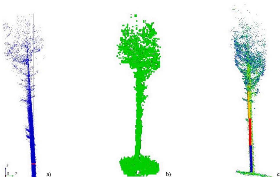
Fig. 5. DBH extraction phases: a) DBH and Tree Height data extracted by 3D Forest; b) Voxelization by “VoxR” package; c) Reconstruction of the geometrical primitives with RANSAC on the points classified as stem.
