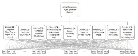
Figure 4. Criteria hierarchical structure to determine the criticality of Kaplan hydro generator unit components (CP).
