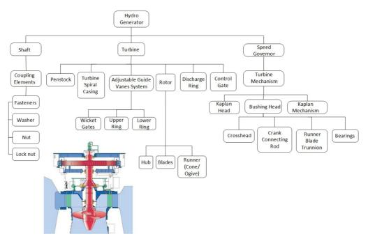
Figure 2. Partial functional tree (FT) of hydro generator Kaplan unit (mechanicals elements).
