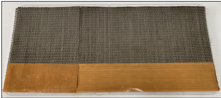
Figure 3.4 – The PTFE film placed in the mid-plane of the preform.
