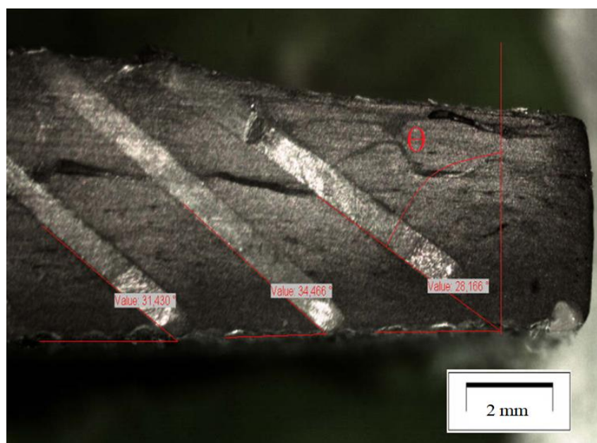
Figure B2 – Z-pins misalignment in the specimen #6.
