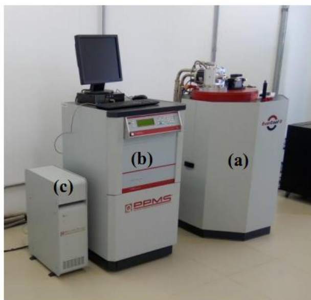
Figure 3.8 PPMS equipment, (a) enclosed superconductor magnetic and the sample chamber, (b) and (c) Human interface and controller system.
