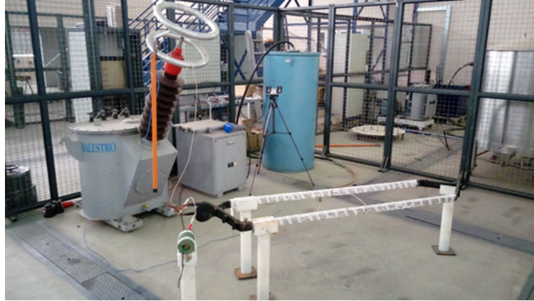
Figure 53 – Voltage Applied - Overview of the Test Configuration
