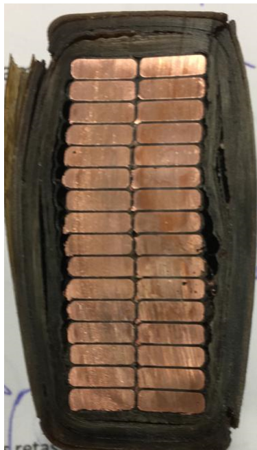
Figure 66 – Thermal cycle test 2 - Insulation breakdown
