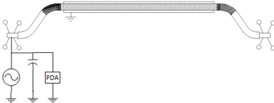
Figure 37 – Detection method for off-line partial discharges measures
