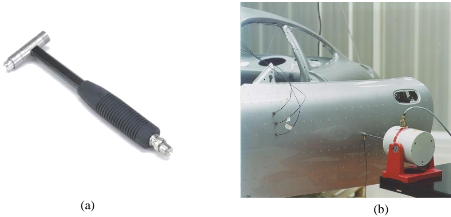
Figure 4.2. Modal analysis. (a) Instrumented hammer used for impact testing. (b) Electromagnetic shaker used to test a car's door with attached accelerometers.
