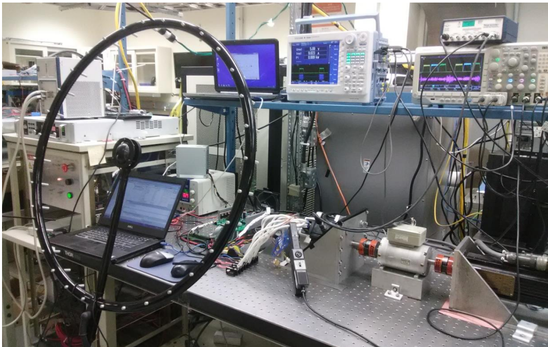
Figure 4.48. Noise measurement using an acoustic camera.
