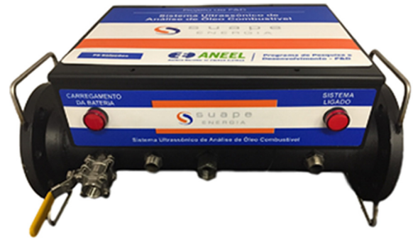
Fig. 9. Field prototype of the proposed ultrasound-based water-cut meter.
