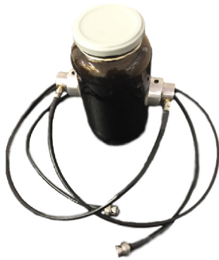
Fig. 5. The glass vessel adapted to the laboratory experiments. Both transducers are placed into the corresponding housings.
