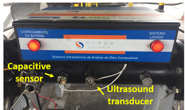
Fig. 14. Capacitive sensor and ultrasound transducer integrated to the field prototype.
