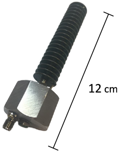
Fig. 12. PCB-based capacitive sensor. Round two-layers PCBs were soldered side by side, forming a particular capacitor.
