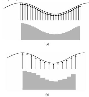
Figure 4. (a) High sampling rate, (b) Low sampling rate
