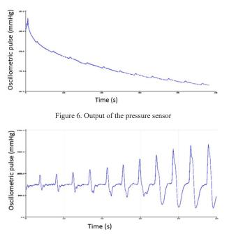
Figure 7. Pressure signal after filtered
