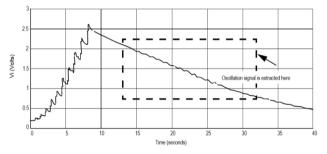
Figure 2. Output signal pressure from sensors
