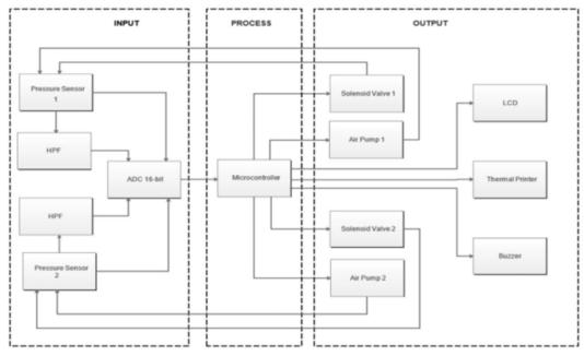
Figure 5. Proposed ABI measurement by Oscillometric Method
