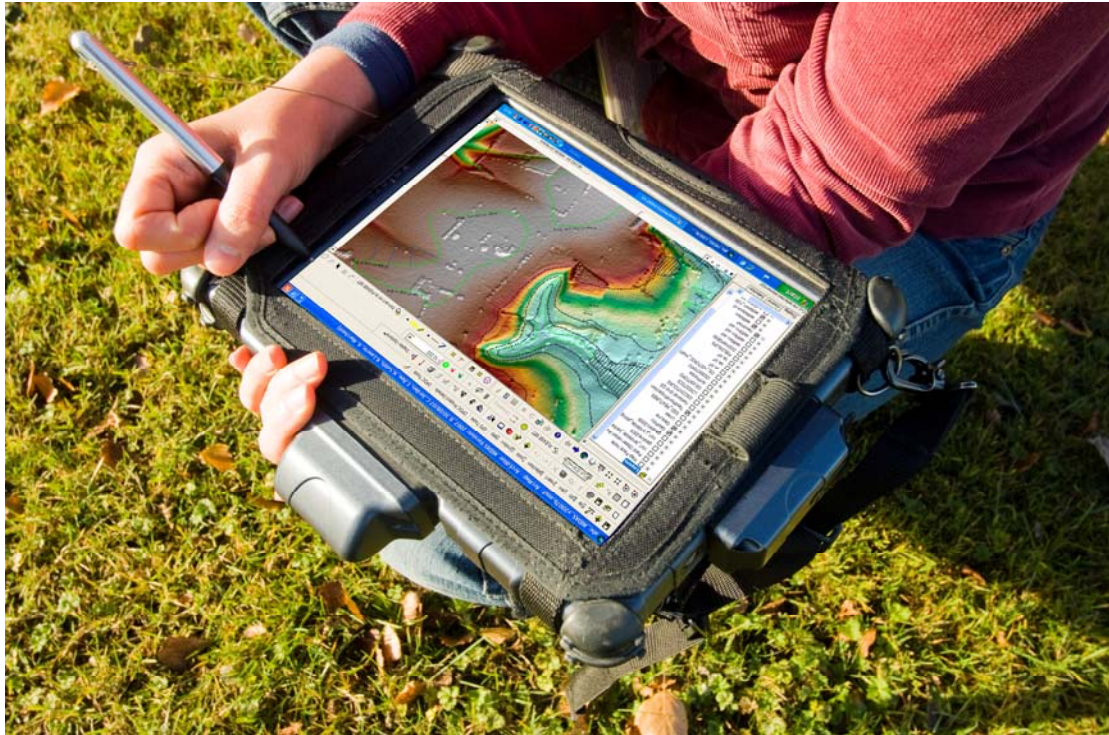
Figure 13. NEXTMap manipulation in the field using a ruggedised tablet PC with integrated GPS, running customised ArcMap Software. Elevation data from Intermap Technologies.
