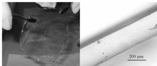
FIGURE 2. Alginate film (on the right, optical microscope image 100 \times ).
