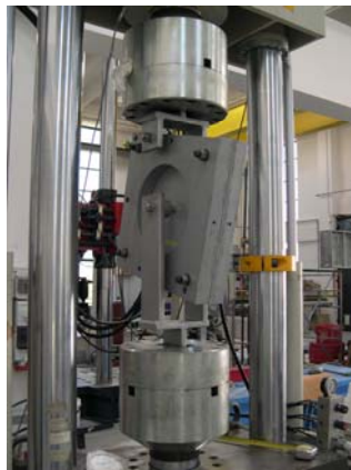
Fig. 4. Fixture attached to Shenck Hydropuls servo-hydraulic testing machine.
