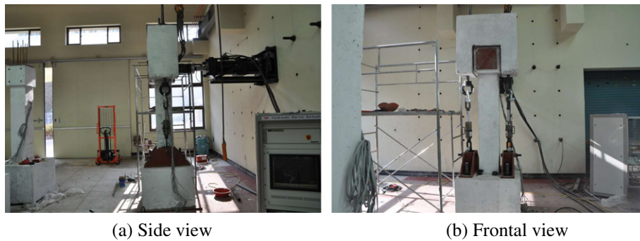
Fig. 8. Setup for cyclic load test of columns.
