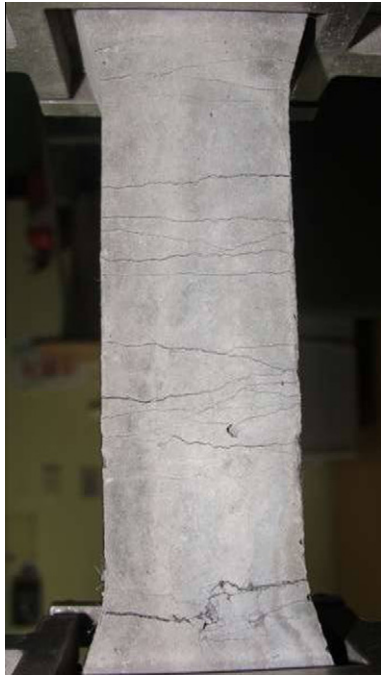
Fig. 5. Multiple micro-cracks of HPFRC specimens.
