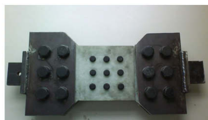
Fig. 8. Double lap bolted joint prototype.
