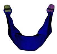
Fig. (9a). Tetrahedral FE mesh of whole temporomandibular joints.
