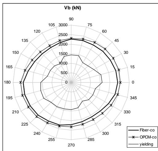
**Fig. 5 - Collapse and Yielding Force-domain for Triangular Distribution**
