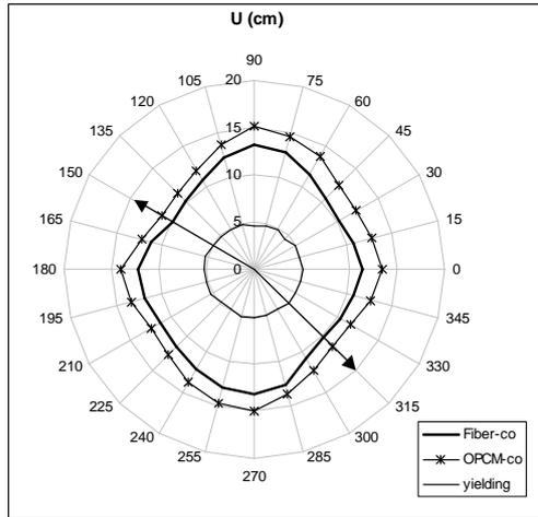
**Fig. 6 - Collapse and Yielding Displacement-domain for Uniform Distribution**
