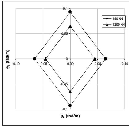
**Fig. 3 – Example of Collapse Curvature Domain for Columns**
