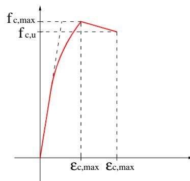
**Fig. 2 - Concrete01: Stress-Strain Relationship**
