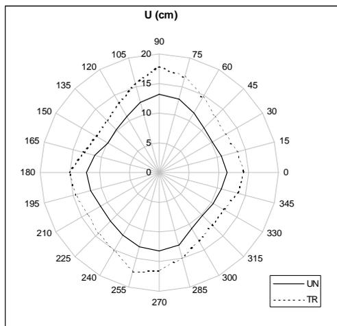
**Fig. 8 - Collapse Displacement-Domain for the Force Distributions under examination.**
