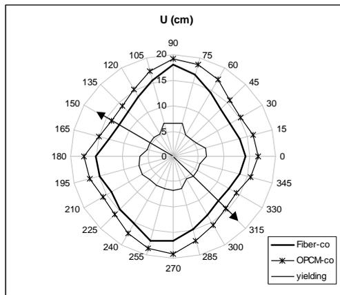
**Fig. 4 - Collapse and Yielding Displacement-domain for Triangular Distribution**
