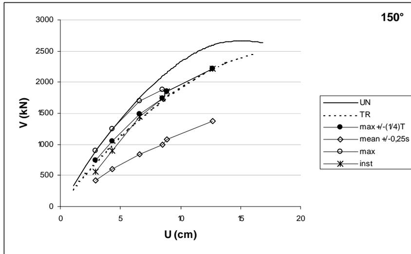
Fig. 15 – Comparison between IDA (*analysis a*) and pushover analyses
