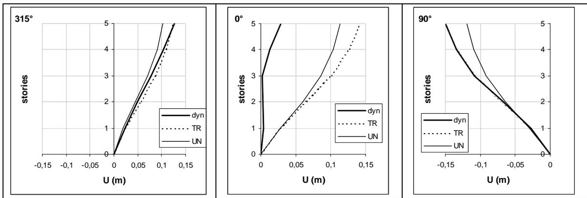
**Fig. 19 - Storey Displacement Comparison at Collapse**
