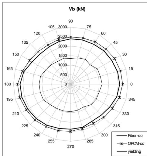
**Fig. 7 - Collapse and Yielding Force-domain for Uniform Distribution**
