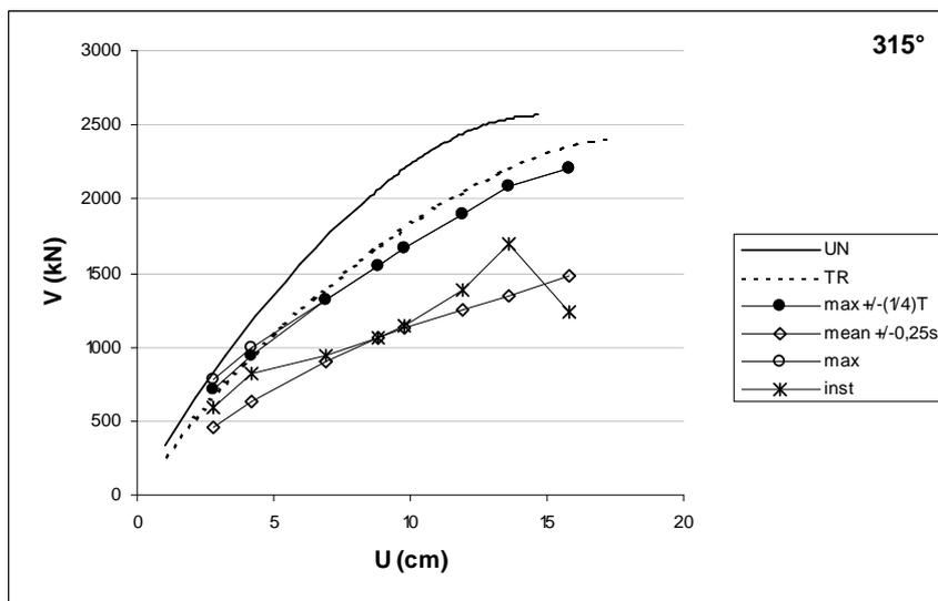
**Fig. 20 – Comparison between IDA (*analysis b*) and pushover analyses**
