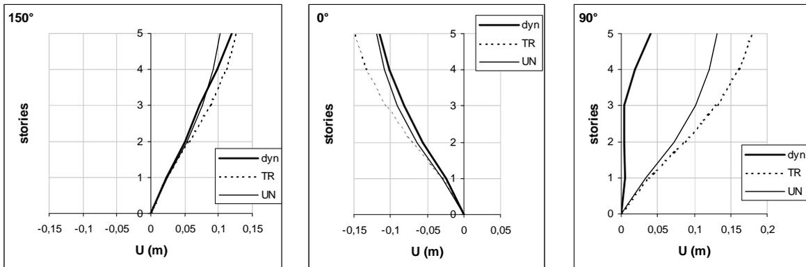
**Fig. 14 - Storey Displacement Comparison at Collapse**
