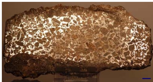
Figure 3. Example of Main Group pallasite Hambleton, displaying areas rich in metal and others rich in olivine.
