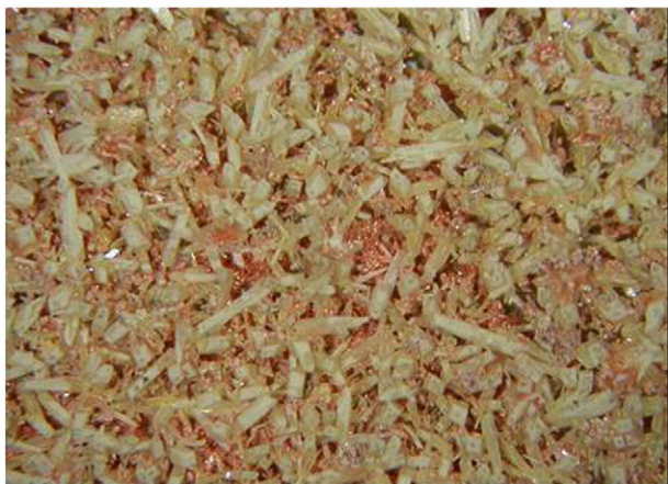
Fig. 10. Simultaneous deposition of metallic copper and cotunnite ( \text{PbCl}_2 ) on the stainless steel cathode.
