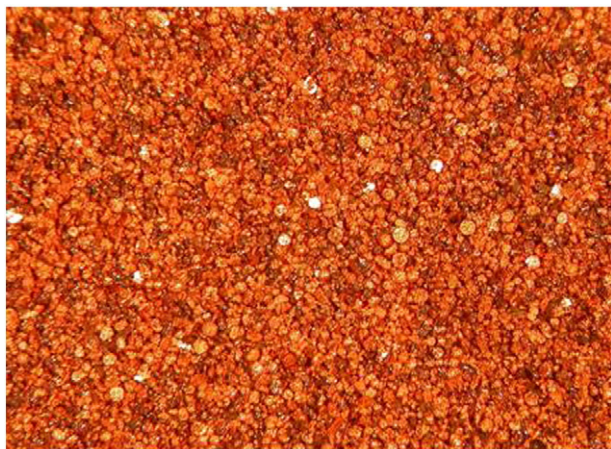
Fig. 4. Small drops of pure copper obtained by cementation onto aluminium film.
