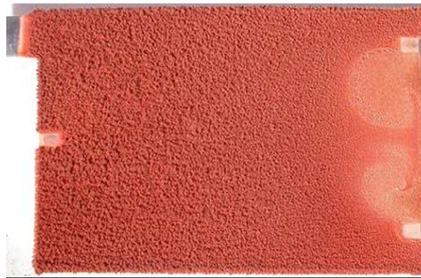
Fig. 8. Stainless steel cathode covered by copper through electrowinning deposition.
