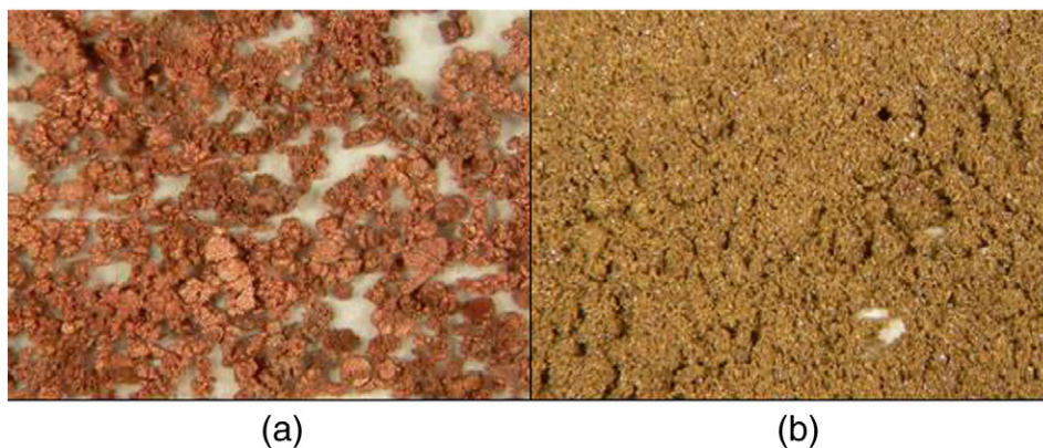
Fig. 1. Cementation products on aluminium as a function of pH: a) copper cemented at pH 3.07, b) nantokite (CuCl) cemented at pH 0.63.
