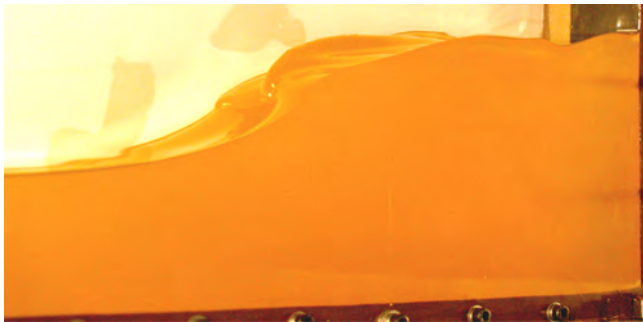
Fig. 18. Lateral impact with oil. 1X. Free surface details.
