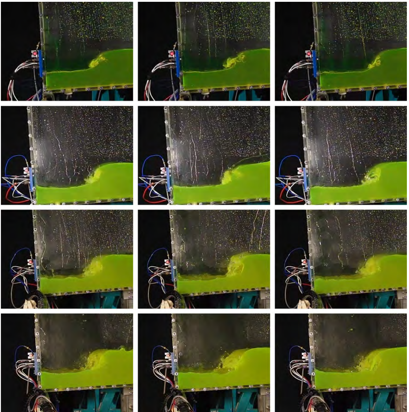
Fig. 6. Lateral impacts with water. Front view sample frames along arbitrarily chosen consecutive cycles for an arbitrarily chosen experiment. Various widths (from top to bottom rows: 0.5X, 1X, 2X, 3X). See supplementary materials at http://canal.etsin.upm.es/papers/soutoiglesiasetaloe2015/ for complete movies.
