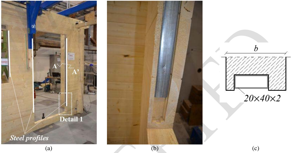
Fig. 4. Specimen HW01 [9]. (a) Overview and position of metal profiles; (b) Detail 1; (c) A-A' cross-section, nominal dimensions in mm.
