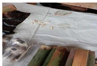
Figure 22. Ulat bumbung when removed from bamboo.
