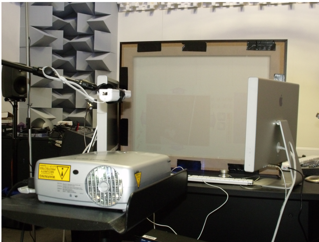
Figure 6.4.7: A view from behind the screen showing the projector and Wii remote.
