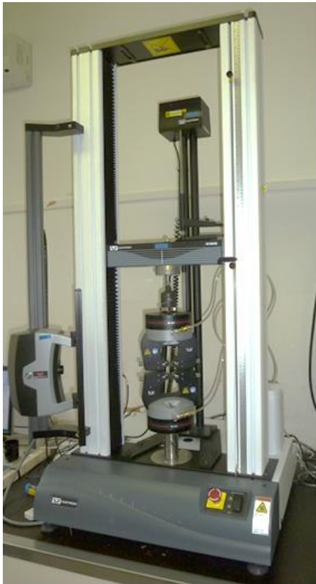
Instron 3366 , software Bluehill 3 Tubes : without extensometer, 50 mm/min, L= 30 mm, 20 pts/s, smooth steel grips 12.5(h)x38(w)mm
