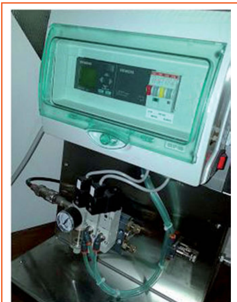
Figure 3. Rear view of instrument: digital control panel and, in the lower left, supply of compressed air provided by a compressor (not shown) used for piston movements.
