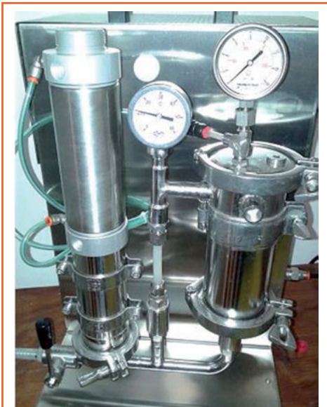
Figure 2. Front view of Estrattore Naviglio®: extraction chamber (right), piston housing (left) and discharge valve (lower left). The instrument allows to constantly monitor pressure (indicator is at upper right) and temperature (left indicator).
