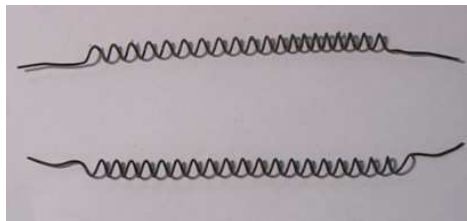
Figure 3 - SMA spring actuator elements.
