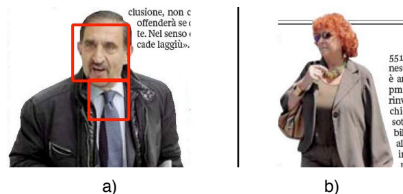
Figure 3: Examples of errors in detection: a) non-relevant error: the false positive on the tie will not find any matching face during recognition; b) relevant error: the missed detection of the face will determine a missed recognition.
