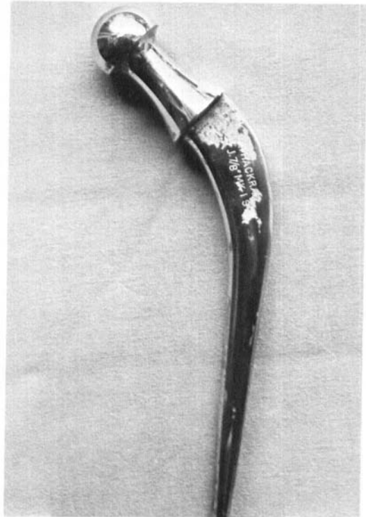
Figure 1. Corrosion pits on the stem of a prosthesis removed after 5 years.
