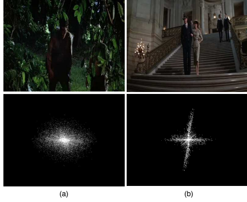
Fig. 6 Examples of global magnitude of the Fourier transform of a) a natural and b) a man-made image (the white plots represent the 80% of the energy).
