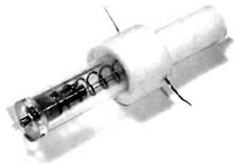
Fig. 1 Picture of the pneumatic mini-valve actuated by the Ni-Ti wires
