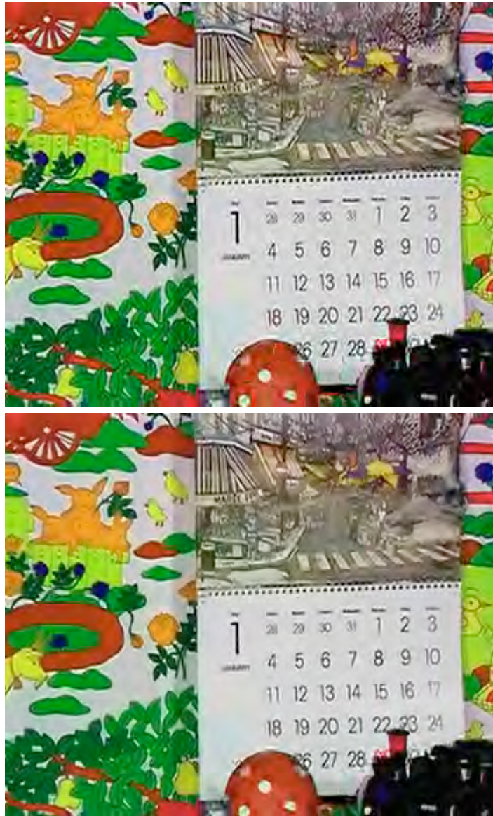
Figure 14 (a)-(c) Visual results with (bottom) and without (top) the use of the de-ringing filter
