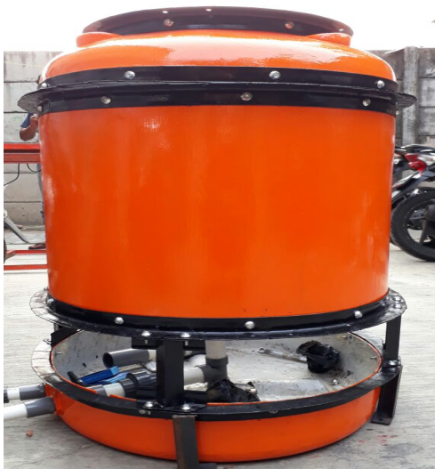
Gambar 5. Tabung Cooling Tower
