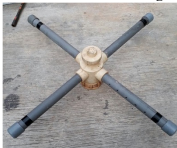
Gambar 7. Sprinkler Cooling Tower
