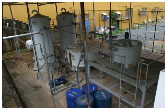
Fig. 1. View of the UFBA biodiesel plant, capacity 10,000,000 \text{ L year}^{-1} .
