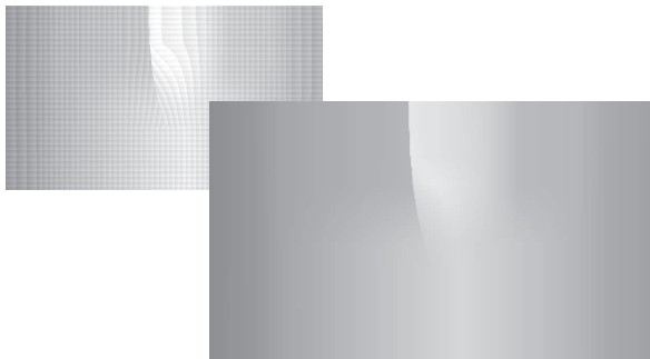
Figure 10: Here, the signal texture is a normal-map encoding a curved surface with a crease. The pinch strength is changed from zero to one over the space of three texels to make the crease start smoothly. Left: texels shown with a superimposed 8 \times 8 grid, right: final result (screenshot).
