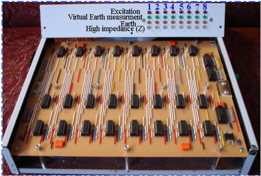
Figure 3-13: A photo of the electrode selection circuit for array A
