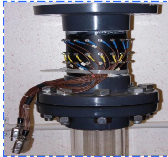
Figure 2-19: Dual plane Electrical Resistance Tomography system
