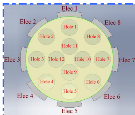
Figure 5-2: Positions of the 12 holes through which the nylon rod was inserted
