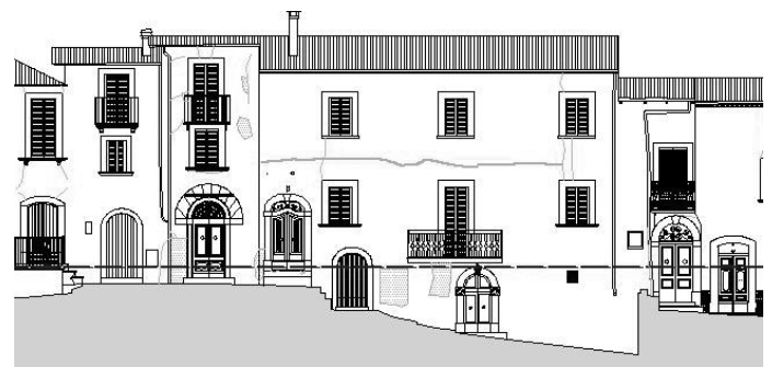
Figure 13: Villa Santa Lucia degli Abruzzi crack pattern.
