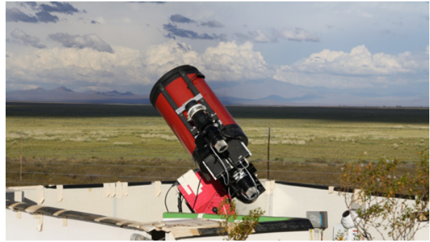
Figure 3. FRAM – F/(Ph)otometric Robotic Atmospheric Monitor is an optical telescope equipped with CCD cameras, and it automatically observes a selected fields of well-calibrated stars.
