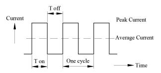
Figure 3 Relation between WEDM input parameters.
