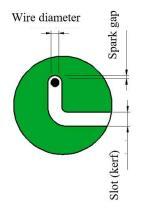
Figure 4 Details of the spark gap in WEDM.
