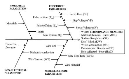
Figure 2 Relation between WEDM input process variables and output responses.
