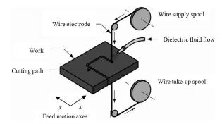
Figure 1 A typical WEDM process.
