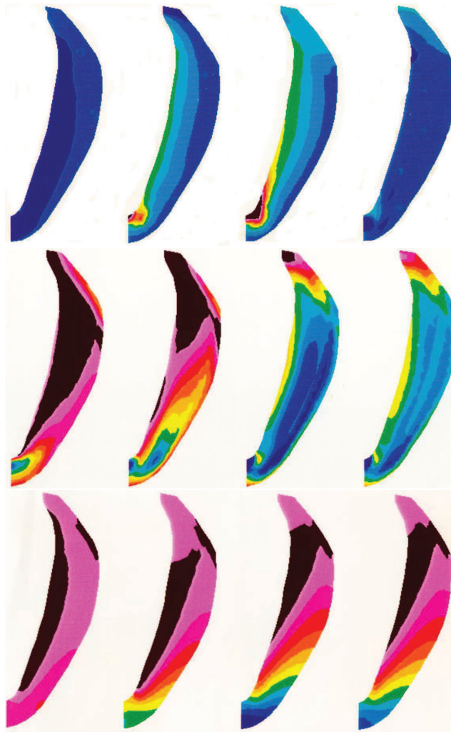
Figure 14: Color coded plots of the intramyocardial pressure (top), sarcomere length (middle) and rotation angle (bottom) of the axisymmetric simulation of the beating left ventricle (Fig. 12). The successive states are from left to right, the end of isovolumic contraction, of ejection, of isovolumic relaxation and of diastole.[HAvCR92]
