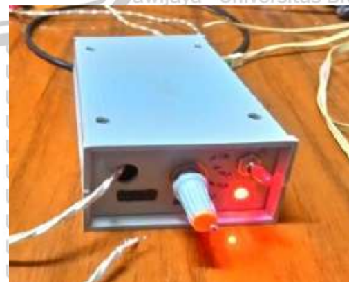
Gambar 12. Converter V to I
