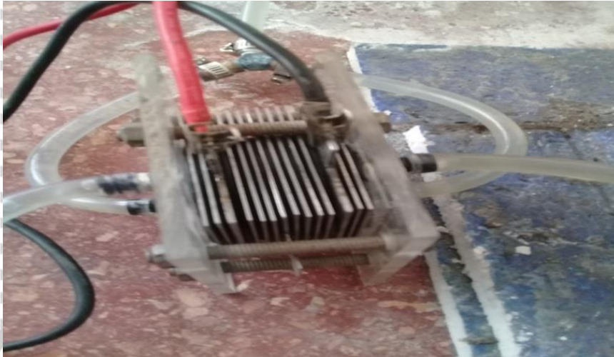
Gambar 2.4 Generator HHO tipe Dry Cell
