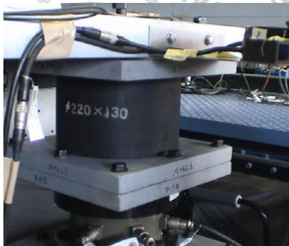
Figure 2. 6 Natural rubber bearing (Taghikhani, et.al., 2005)
