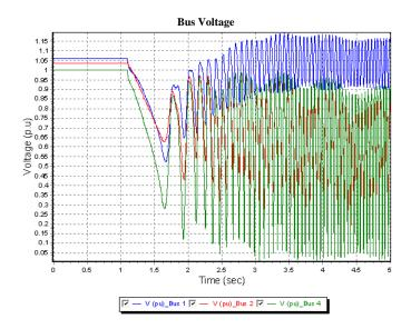
Figure 4. Bus-voltage at loss two transmission lines both end
