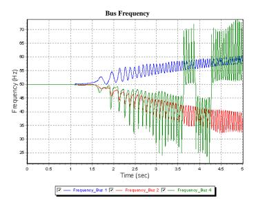
Figure 5. Bus-frequency at loss two transmission line both ends
