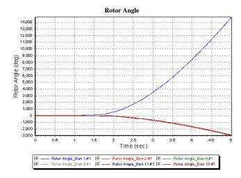
Figure 3. Show rotor angle at loss two transmission lines both ends
