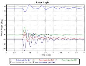
Figure 6. Rotor angle at three phase fault
