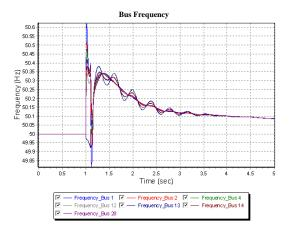
Figure 8. Bus-frequency at three phase fault
