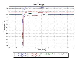
Figure 7. Bus-voltage at three phase fault
