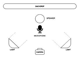
Figure 1. Audio-visual Equipment Setup for Javanese Emotion Database Recording
