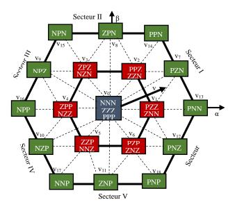
Figure 2. Voltage vector distribution of the 3-level NPC inverter
