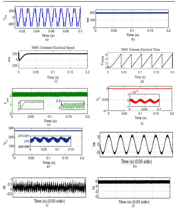
Figure 5. a) Inverter voltage, b) speed, c) observed speed, d) observed electrical angle, e) electromagnetic torque  $T_{em}$ , f) the neutral point voltage  $V_z$ , g)  $V_{c1}$ , h)  $i_a$ , i)  $i_d$ , j)  $i_q$  at  $T_r = 2 \text{ N.m}$
