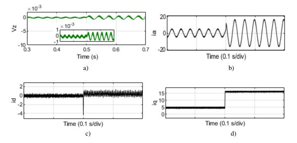
For a load torque varying from 2 to 6 N.m in 0.05 s, figure 7 shows the results obtained.
