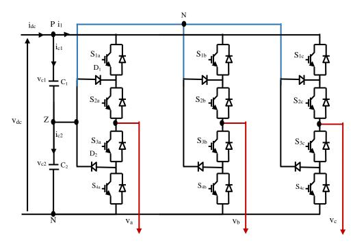
Figure 1. 3-phase NPC 3-level inverter
