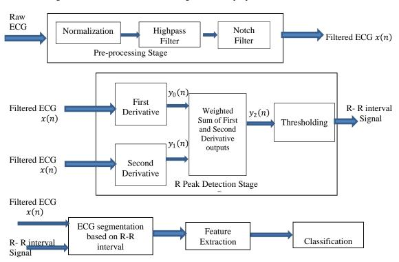
Figure 2. Detailed block diagram of the proposed technique
