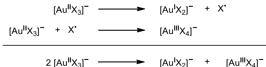
Scheme 1.12. Disproportionation process undergone by the [\text{AuX}_3]^- anions. Disproportionation enthalpy values ( \Delta H_{\text{dis}} ) are as follows: \text{X} = \text{F} , -186 \text{ kJ mol}^{-1} ; \text{X} = \text{Cl} , -132 \text{ kJ mol}^{-1} ; \text{X} = \text{Br} , -103 \text{ kJ mol}^{-1} ; \text{X} = \text{I} , -74 \text{ kJ mol}^{-1} .
