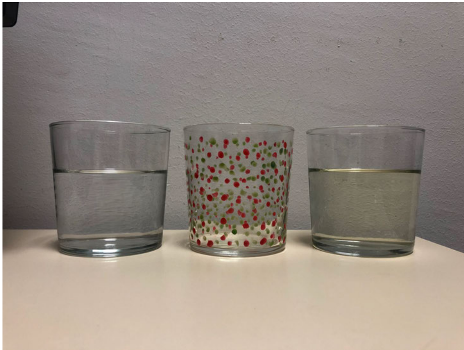
Figure 3.1: Containers used for simulation, representation and comparison with the virtual phantom. The three glasses are identical. The middle glass will be virtually filled with the replica of the liquid volume. Since it is empty, the painted texture helps the cameras to track its movement.
