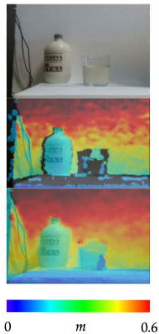
Figure 4.9: Color and depth stream before (up) and after (down) applying filters to reconstruct the depth map
