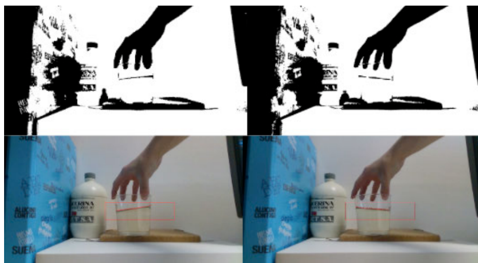
Figure 4.10: Representation of the color frame and its conversion to a binarized image to seek the free surface. The area defined for searching is represented in the color frame as well as the points of the free surface detected in the black and white image.
